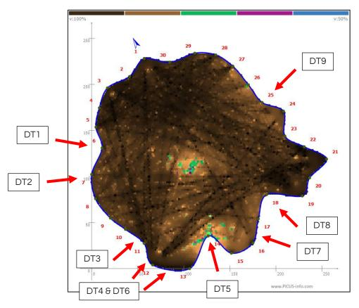
To confirm the tomogram, the Resi PD400 was used in nine locations at the level of assessment – please see the drill traces below:
