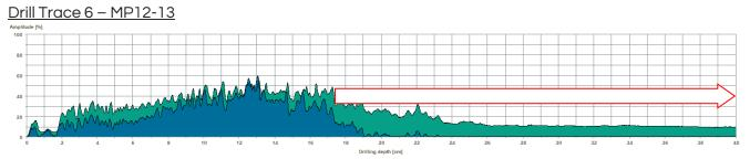
• The drill trace indicates an area of extensive decay forming from c.17.5cm through to the end of the assessment
