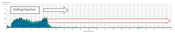
• (Please note, historically Resi drill traces have read from right-to-left due to the configuration of the original machine. However, by using the software available, I have flipped the drill traces to read left-to-right, the more conventional way to read a graph)
